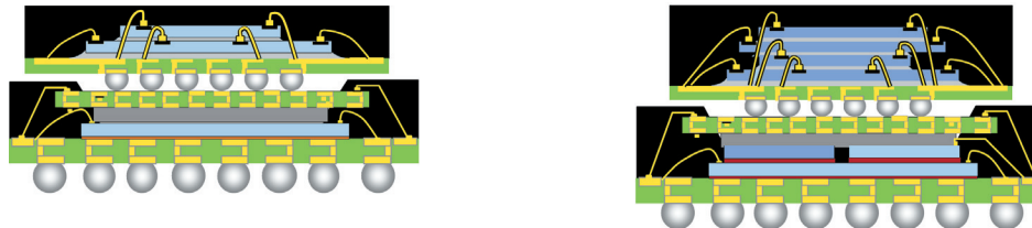
Assembled FiPoP Package Solutions (with top and bottom package)
